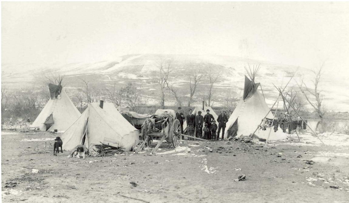
The versatility of the cart was unmatched. With its high wheels, the cart could transverse the rutted prairie, be disassembled and floated as a raft across streams, or covered with waterproof hide and transformed into a boat. The wheels were simply removed and lashed to the bottom to form a raft. At day's end, the cart could then be both covered with
